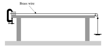
Add to the diagram suitable apparatus for measuring the extension of the wire as further masses are added to the slotted hanger.
