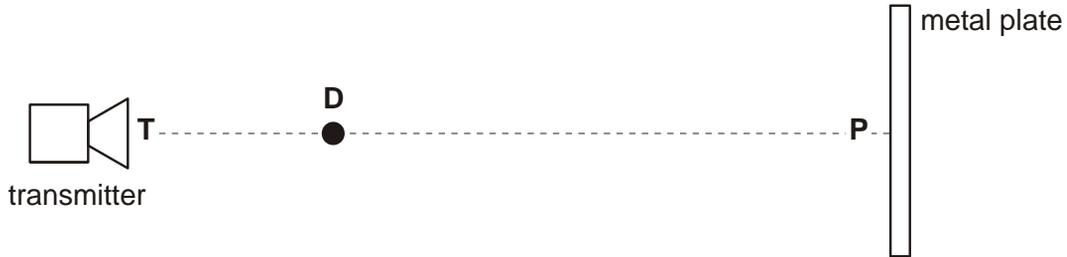
Microwaves leave the transmitter and move in a direction **TP** which is at right angles to the metal plate. A standing (stationary) wave is formed between **T** and **P**.
