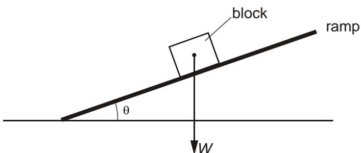
The angle between the ramp and the horizontal is  $\theta$ .
