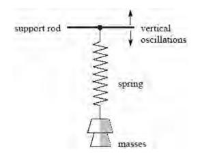
The response of the masses suspended from the spring to the vertical oscillations of the support rod varies with frequency. Describe and explain, as fully as you can, the motion of the masses when the support rod oscillates at a frequency of (i) 0.2 Hz, (ii) 1.5 Hz and (iii) 10 Hz.
