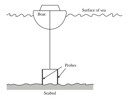
Taking measurements using these probes, resistivity can be calculated at various depths below the seabed.
