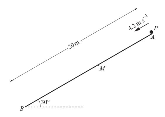
A and B are points at the upper and lower ends, respectively, of a line of greatest slope on a plane inclined at 30° to the horizontal. The distance AB is 20 m. M is a point on the plane between A and B. The surface of the plane is smooth between A and M, and rough between M and B.
