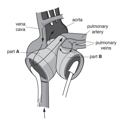
(a) Part A and part B in the artificial heart pump blood to different places.
