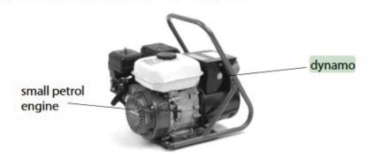
The small petrol engine drives the dynamo. The dynamo generates electricity. This arrangement is not efficient in generating electricity.
