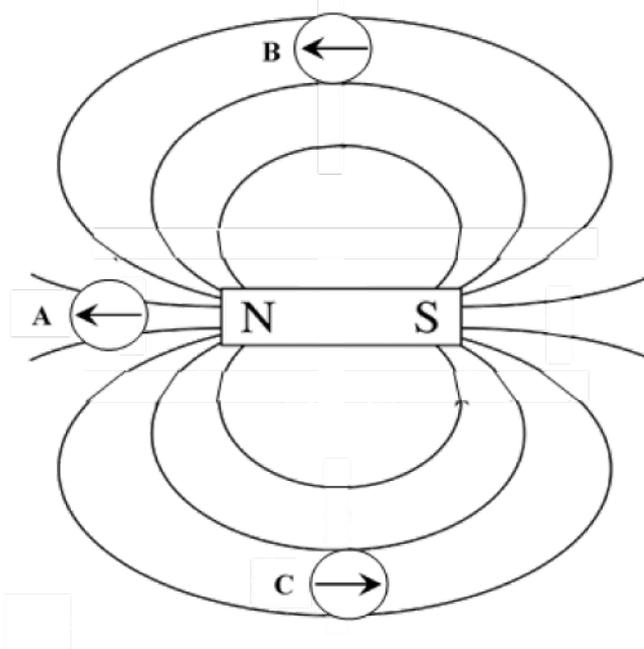
(i) Which of the plotting compasses, A, B or C, is faulty and pointing in the wrong direction?
