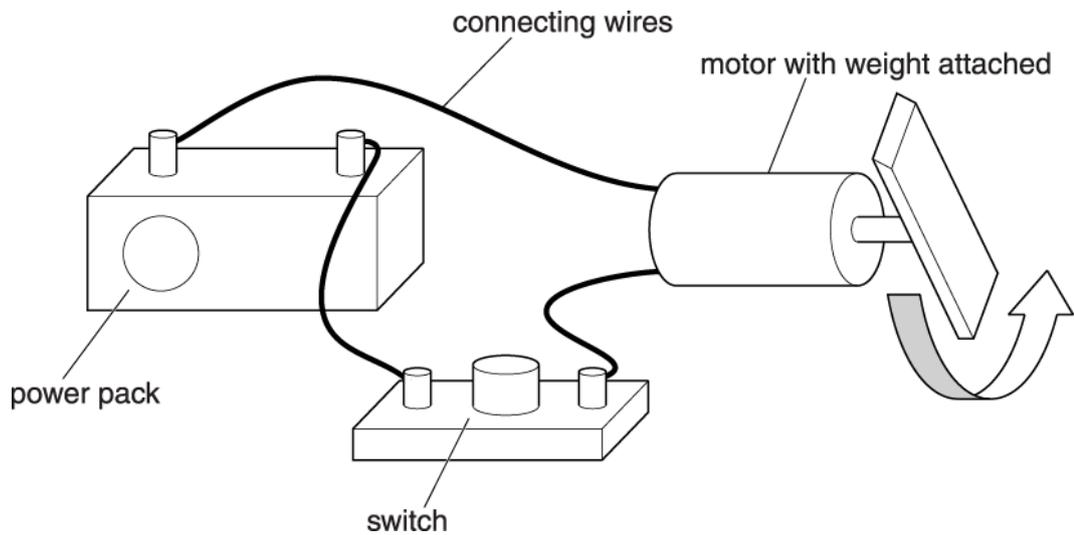
When Luke turns on the circuit, the motor rotates.
