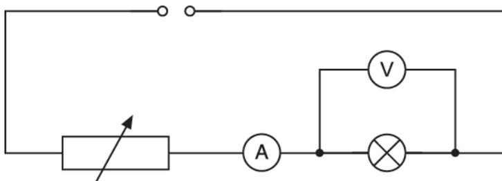
(i) On the diagram put a **ring** around the symbol for the ammeter.
