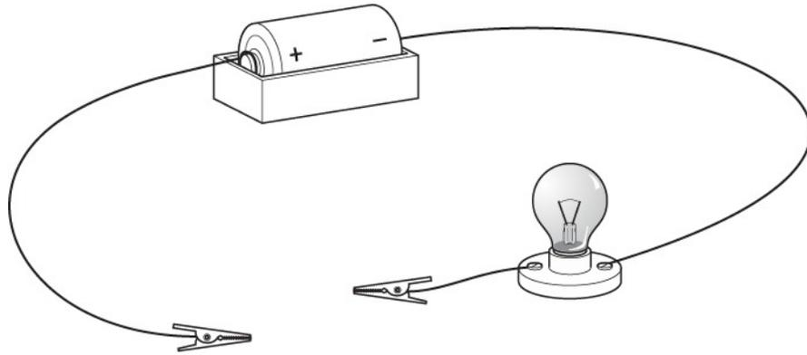
The lamp glows when she puts a piece of copper into the circuit between the clips.
