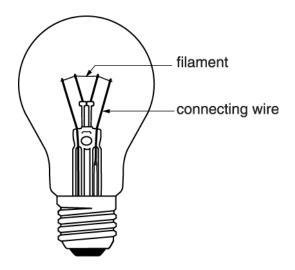
The filament wires in the lamp are much thinner than the connecting wires.
