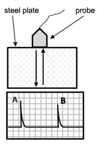
The probe sends out a sound wave into a sample of steel plate.
