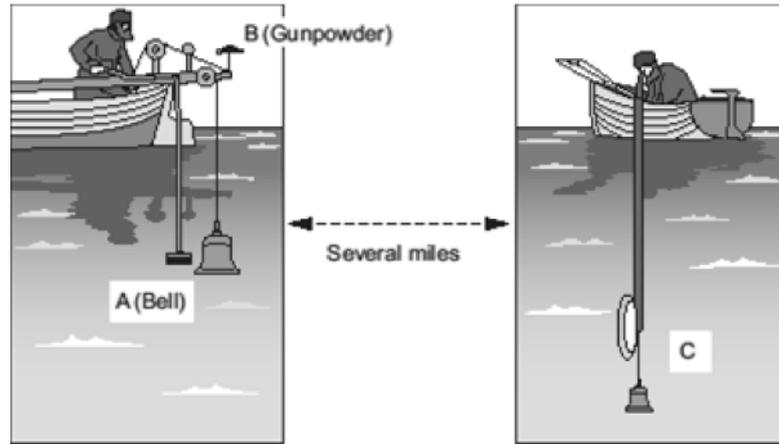
The bell (A) was struck and the gunpowder (B) ignited at the same time. The flash from the gunpowder and the sound from the bell were picked up several miles away (C).
