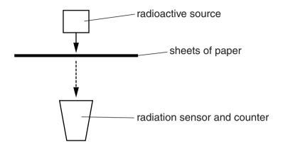
Dr Williams measures the nuclear radiation from each source using the sensor. Each radioactive source emits only one type of radiation.
