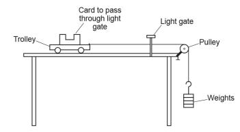
The trolley is released from a fixed position and accelerates.
