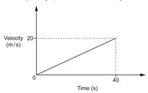
Acceleration is the gradient of a velocity-time graph.
