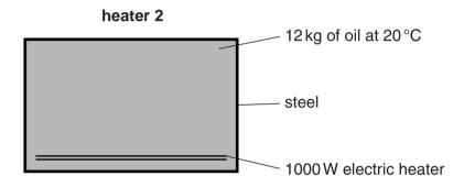
Heater 1 is filled with water. Heater 2 is filled with oil.
