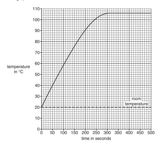
Write down the time interval during which **all** of the energy supplied was used to change the state of the liquid, and explain how the energy supplied causes this change of state.
