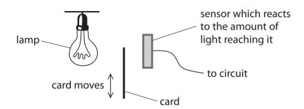
The piece of card can be moved up and down between the lamp and the detector. Each part of the teacher's arrangement corresponds to a part of the machine.
