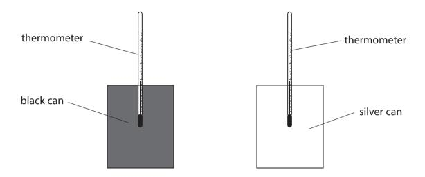
Hot water is poured into the cans and the temperature of the water in each can is measured every two minutes.
