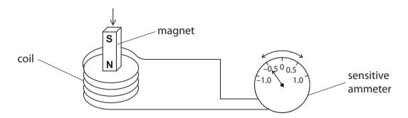
The moving magnet and the coil of wire are producing an electric current.
