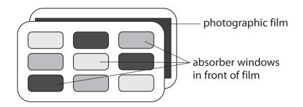
Each absorber window is made from different thicknesses of paper, aluminium or lead.
