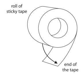
This causes both the roll and the end of the tape to become electrically charged by friction.
