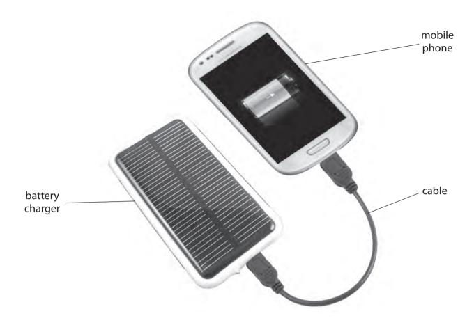
When the battery charger is used, it transfers light energy from the Sun to the battery of the mobile phone.
