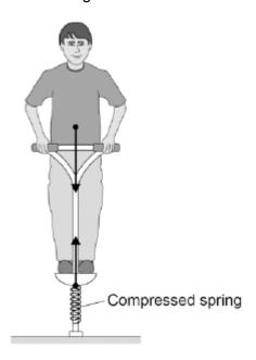
(a) The downward force of the child on the spring is equal to the upward force of the spring on the child.
