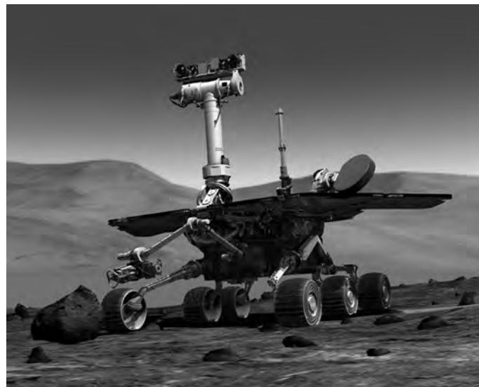
The Mars Rover has a mass of 185 kg.
