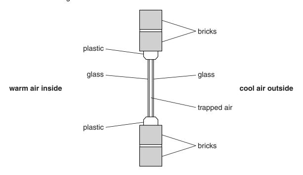
The energy from the warm air inside is transferred through the double glazing to the cool air outside.
