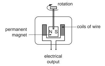
A voltage is produced when the magnet rotates.
