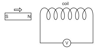
The voltmeter gives a reading when the magnet is moving.
