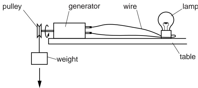
When Rai lets the weight fall, the generator spins and the lamp lights up.
