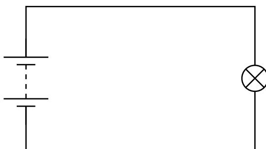
Add a voltmeter to the circuit diagram to show how the voltmeter should be connected to measure the voltage across the battery.
