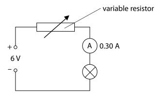
(i) The current in the lamp is 0.30 A. Calculate the charge flowing through the lamp in 30 seconds. State the unit.
