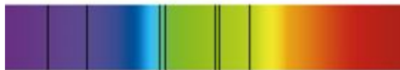
Absorption spectrum showing the absorbed frequencies as thin black lines (adapted from circlingsquares.blog).
