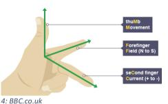
Force on a current-carrying conductor can be calculated as followed: F = BIL
