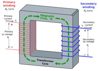
• Fewer coils on secondary: Step down transformer, as smaller PD induced on secondary
