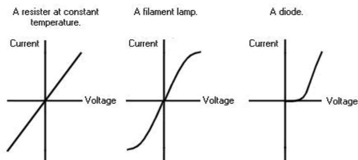
*inteleducationresources.intel.co.uk – gradient of each is  $1/\text{resistance}$ , so a sharper gradient means a lower resistance*
