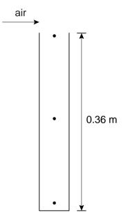
The length of the tube is 0.36 m. The air column in the tube is sounding its lowest (fundamental) frequency note.
