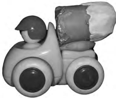
A student carries out an experiment to find the speed of a pellet fired from an air rifle. The pellet is fired horizontally into the modelling clay. The pellet remains in the modelling clay as the car moves forward. The motion of the car is filmed for analysis.
