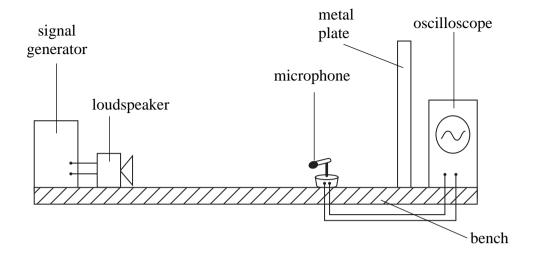
A loudspeaker is connected to a signal generator. A microphone is connected to an oscilloscope. Sound waves reach the microphone directly from the loudspeaker and after reflection from the metal plate.
