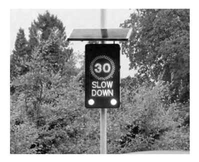
The speed of an approaching car is measured by transmitting microwaves towards it. These waves are reflected off the car and picked up by a receiver, which uses the Doppler effect to calculate the speed of the car.
