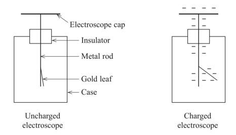
A gold leaf electroscope can be used to demonstrate the photoelectric effect. A clean zinc plate is placed onto the cap of the electroscope and the plate and electroscope are charged negatively. Ultraviolet radiation is shone onto the zinc plate.
