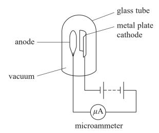
When light is incident on the cathode, the microammeter shows a current.
