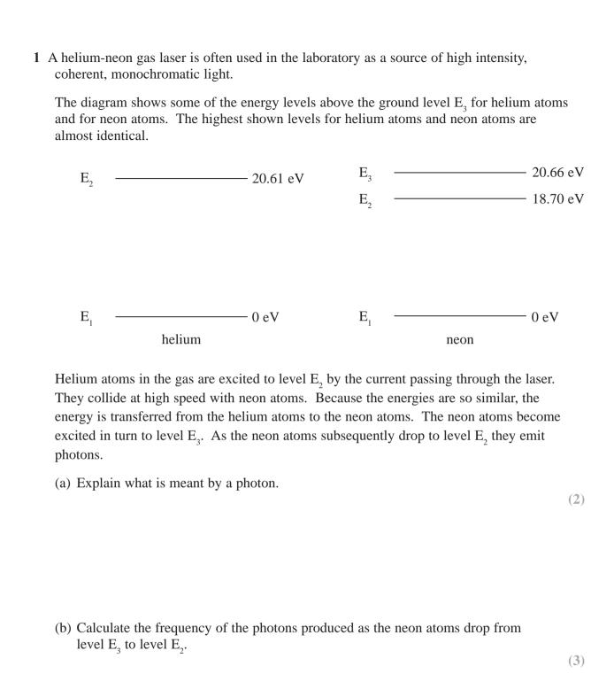
(c) An electron in level  $\rm E_3$  of neon has 0.05 eV more energy than an electron in level  $\rm E_2$  of helium.
