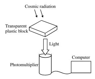
Cosmic radiation causes this plastic block to emit light. If this light enters the photomultiplier, photoelectrons are released and the signal is sent to a computer which records the event.
