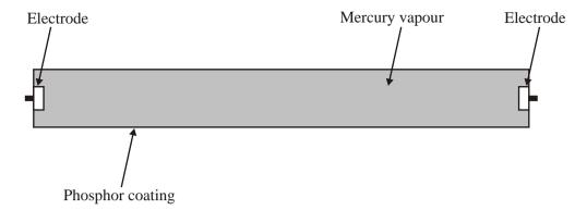
When the tube is switched on a charge flows between the electrodes and the mercury atoms become excited. The mercury atoms then emit radiation.
