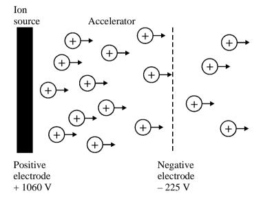
Atoms of xenon are ionised and then accelerated until they are ejected out of the rear of the probe, providing the means of propulsion.
