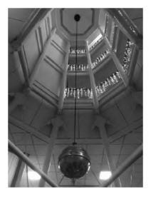
This is a pendulum that consists of a massive sphere, suspended by a long wire from a high ceiling. Over time the vertical plane through which the pendulum swings appears to rotate because of the rotation of the Earth.
