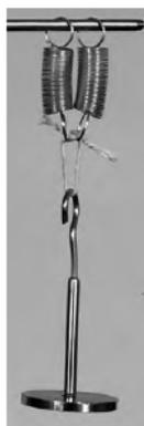
What is the total strain energy stored with two springs arranged in this way?
