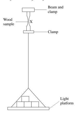
The wood sample is clamped securely to a supporting beam. A light platform is suspended from the wood sample using another clamp.
