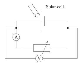
The student keeps the intensity and wavelength of the incident light constant and adjusts the variable resistor to obtain the following set of results.
