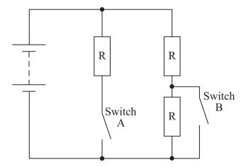
The table gives the four possible combinations of the two switches. Complete the table to show the total circuit resistance for each switch combination.
