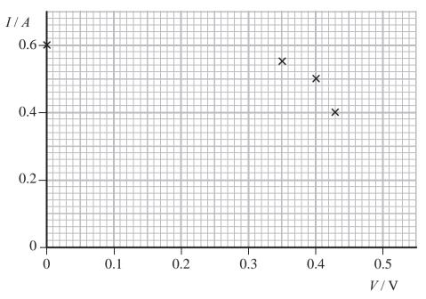
(b) (i) Calculate the power output of the solar cell when the current in the cell is  $0.40\,\mathrm{A}.$
