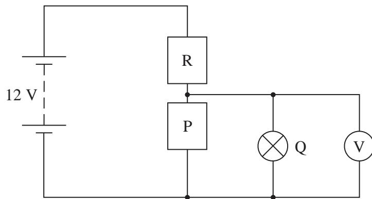
The supply has a negligible internal resistance. The reading on the voltmeter is 4.0 V.
