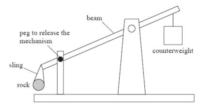
The rock is held in a sling. When the peg is removed the counterweight falls and the rock is projected through the air.
