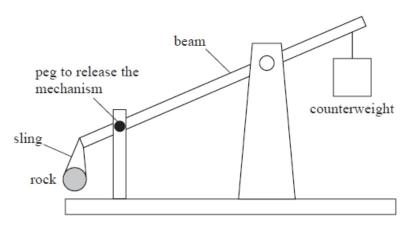
The rock is held in a sling. When the peg is removed the counterweight falls and the rock is projected through the air.
