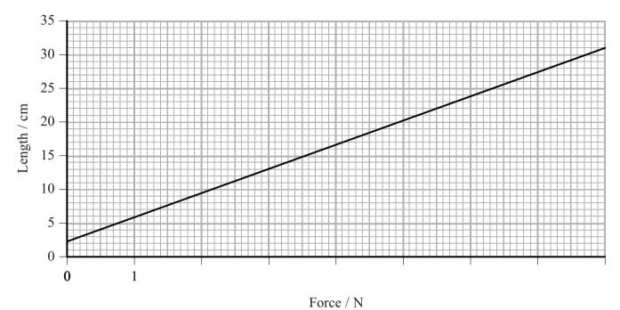
(a) The student concludes that the spring does **not** obey Hooke's law because the line does not pass through the origin.
