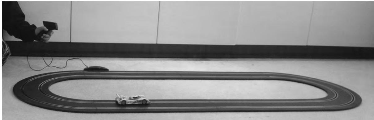
A child places a car of mass 95 g on the track. She adjusts the controller to a power of 4.2 W so the car accelerates from rest for 0.40 s.
