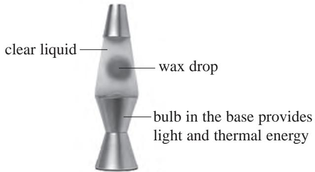
When the lamp is switched on, large drops of liquid wax are seen to rise and then fall within the clear liquid.
