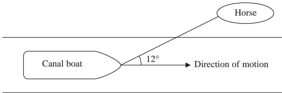
A horse is pulling a canal boat using a rope at  $12^\circ$  to the direction of motion of the boat. The tension in the rope is 1150 N.
