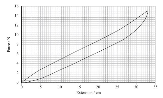
The graph produced by the student shows the stretching force against extension for the elastic waistband. The top line was recorded as the force increased and the lower line as the force decreased.
