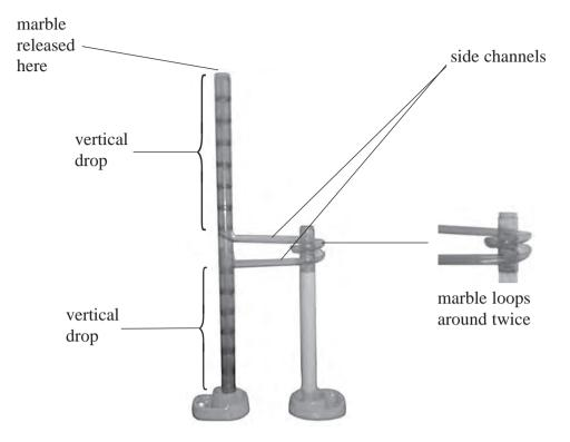
A marble was released and its motion was recorded using a digital video camera. The data was uploaded to a computer and then analysed using a motion capture programme. The following vertical displacement-time graph was obtained.
